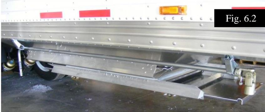
3. Locate the universal joint and roll tube spline on the tarp roll tube, rear of the trailer.
