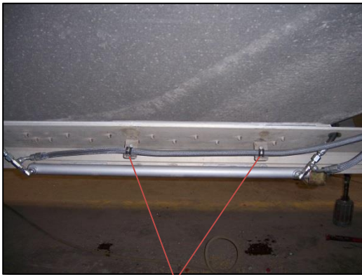
029-51077 – hydraulic hose bracket, 2 per trap frame rail on curb side only.
