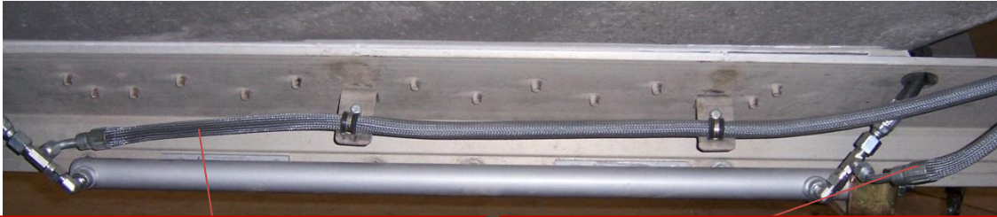
Rear hopper 029-51087 – 132” hydraulic hose. End with 90 degree fitting attaches to cylinder rod end.
