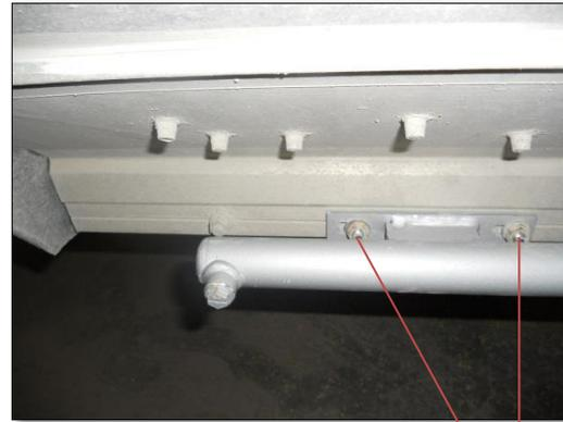
Install hydraulic cylinders with the 3/8" X 2 bolt – washer – roller – washer – washer – trap frame – cylinder foot – washer – nut.
