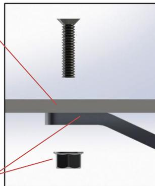
Clamp the door bracket and the reinforcing angle together and secure with 3/8" x 1 1/4" bolts and nuts. If necessary drill holes in bottom lip of the door bracket using the reinforcing angle as a guide.
