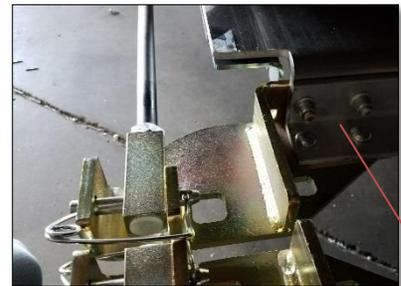
Clamp door bracket to the front lip level with the edge of the door. Drill 13/32" holes in center of each slot.
