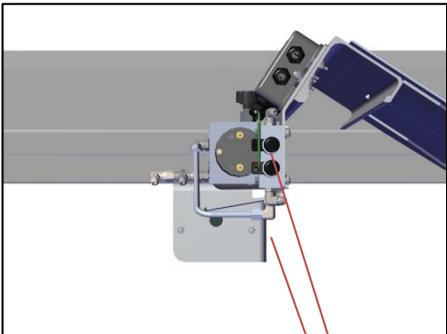
Line up leading edge of bracket with the hydraulic pump mount bracket.
