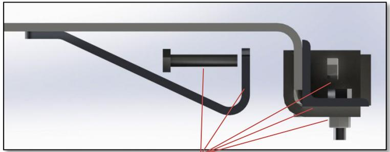
Attach reinforcing bracket, and the door bracket to rear lip of the door and the reinforcing angle to the front lip of the door with 3/8" x 2 bolts and nuts on both sides. Finish attaching the door brackets using 3/8" x 1 1/4" bolts and nuts.
