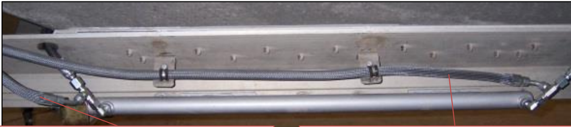
Front hopper 029-51239 – 104” hydraulic hose. End with 45 degree fitting attaches to cylinder rod end.
