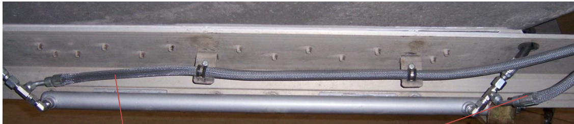
Rear hopper 029-51459 – 197” hydraulic hose. End with 90 degree fitting attaches to cylinder rod end.
