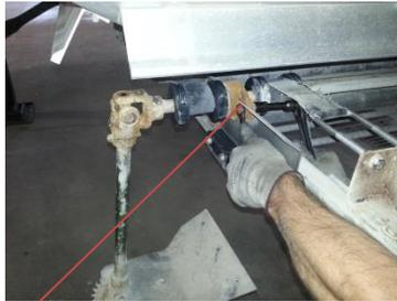
Four bolts per door opener shaft (two per side) to be removed.
