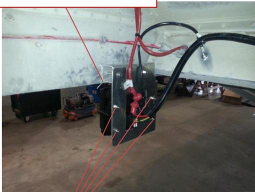
Mount control box with 1/4" bolts and 1/4" nylock nuts.
