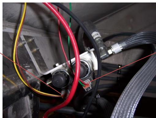
Connect the plug with red/green wires of wiring harness 031-50470 to the upper valve on the hydraulic blocking valve.
