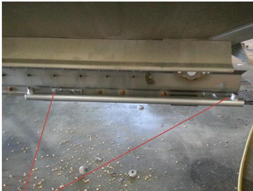
Hold hydraulic cylinders with the 3/8" X 1 1/2" bolt
