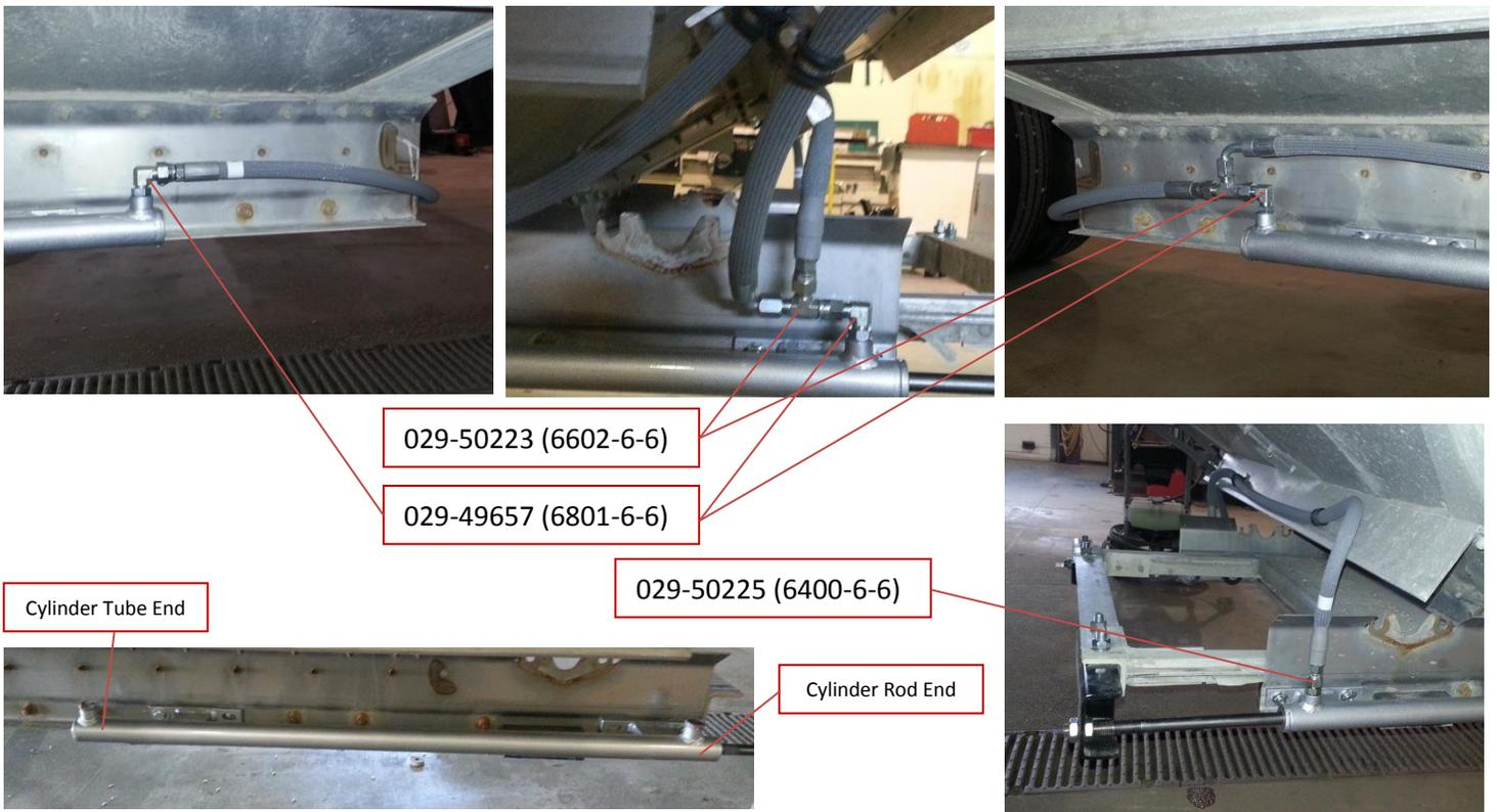
d. Hydraulic pump and blocking valve fittings.
