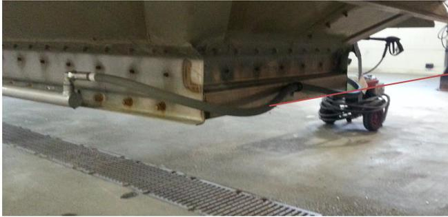
Use 029-53991 – 56-1/2” hydraulic hose. Hose goes across hopper to other cylinder. Use clips to mount as shown. Rear of hopper, cylinder tube end
