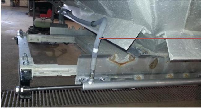
Use 029-53989 – 46-1/2” hydraulic hose. Hose goes across hopper to other cylinder. Use clips to mount as shown. Front of hopper, cylinder rod end
