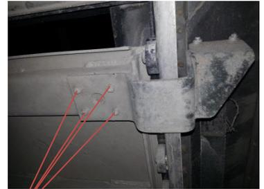
Four fasteners per rear strap bracket (two per side) to be removed.
