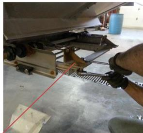
Two bolts per front strap bracket to be removed.
