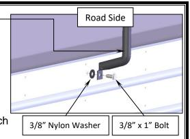
If the interior is accessible, use the bolt, nylon washer, and nut as shown to attach the strap.
