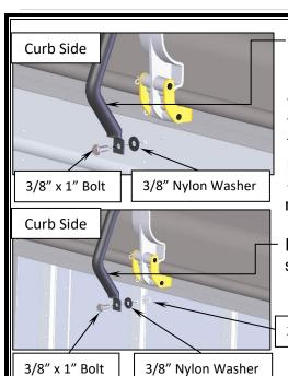
Drape the Thunder Strap tarp keeper strap over the closed tarp. Install the fasteners on the curb (passenger) side of the trailer to hold the straps in place. If the interior is not accessible use the bolt and nylon washer as shown to attach
