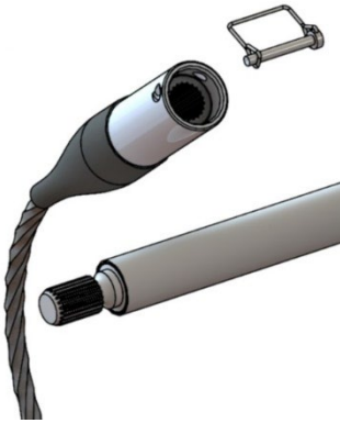
Figure 5. Roll tube spline, coupler and retaining pin shown
