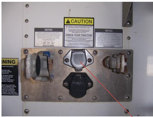
031-51223 – 2 pole vertical receptacle placement
